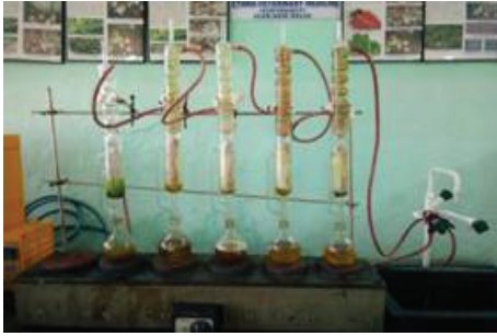
Fig.3. Soxhlet extraction and powder preparation of CQ
