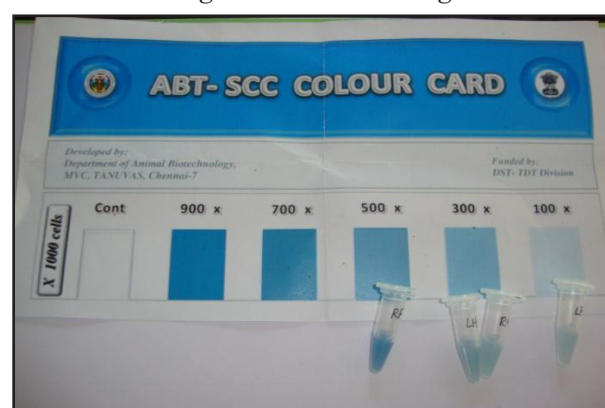
Fig : A TANUCHEK SCC TEST - Colour developed by the test is compared with the score card
