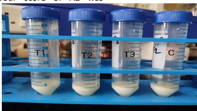
Figure 2: Ultrasonication at different durations - Image showing emulsion stability of spread at different durations (T 1 - 10 minutes, T 2 - 20 minutes, T 3 - 30 minutes for 30% amplitude, C- Without ultrasonication)
