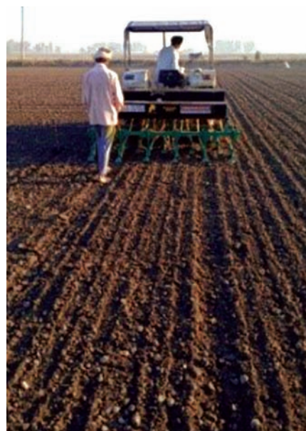
Fig. 6. View of Direct seeded rice drill in operation which was provided to farmers of various blocks of Jalandhar by Krishi Vygyan Kendra, Jalandhar
