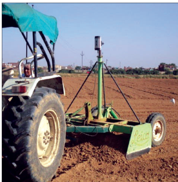
Fig. 1. Laser assisted leveling
