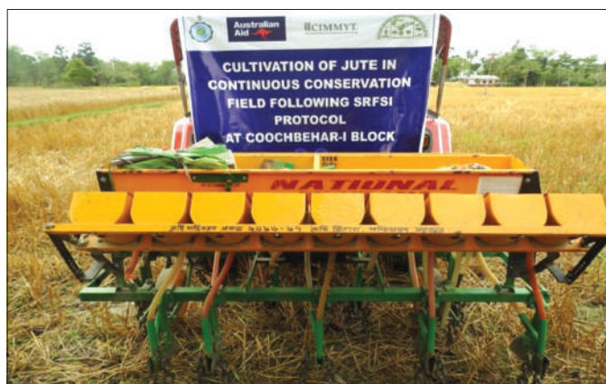
Fig. 2. Jute sowing through multi crop planter in wheat residues
