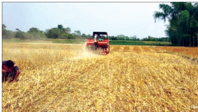
Fig. 1.a. Jute sowing through happy seeder in wheat residues
