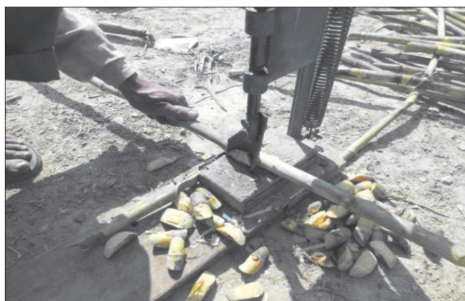
Cutting of bud chips by using bud chipping machine
