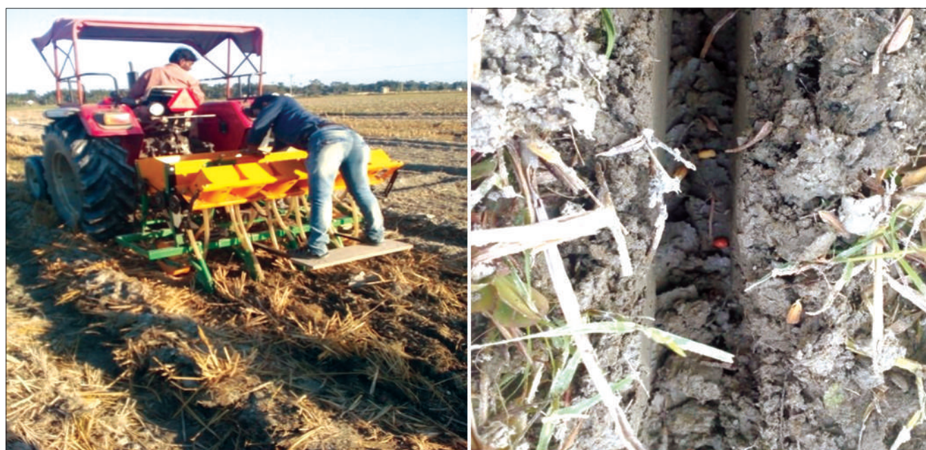
Fig. 1. Zero till fertilizer-cum-seed drill sowing of wheat (left) and opened furrow with placed seed and fertilizer (right)
