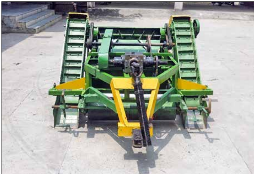
Developed tractor-operated seeder for mat type paddy nursery
