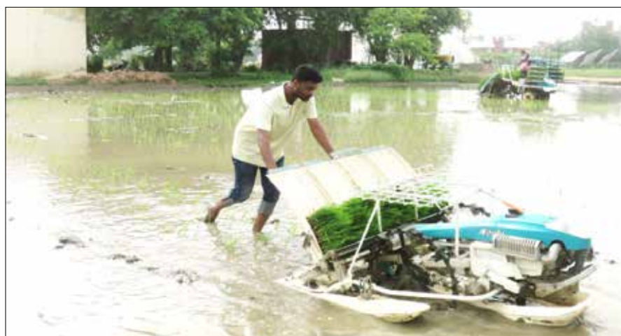
Mechanical transplanting of rice using mechanically grown nursery
