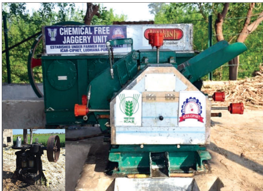
Modern Horizontal crusher. (Inset) Traditional vertical crusher.
