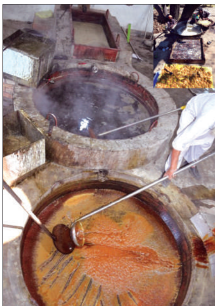
Modern method of jaggery concentration using three pans. (Inset) Traditional method of jaggery concentration using single pan.
