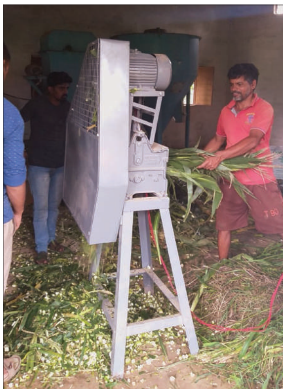
Chaff cutter installed at milk society.
