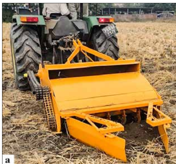
Developed Turbo bund former (a) and working view of the machine (b)
