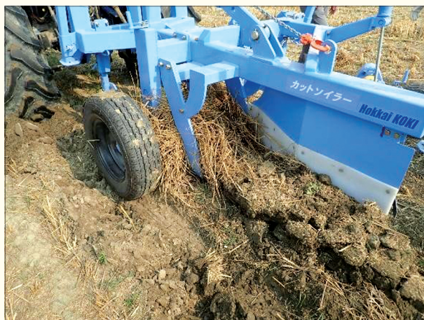
Cut-soiler working under field condition and pearl millet crop
