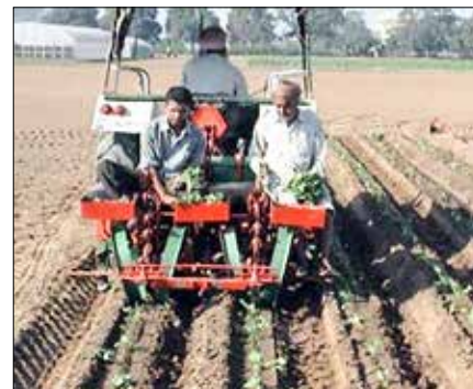
Tractor drawn semi-automatic vegetable transplanter for vegetable seedlings developed at Punjab Agricultural University, Ludhiana (left) and Maharana Pratap University of Agriculture and Technology, Udaipur (right)
