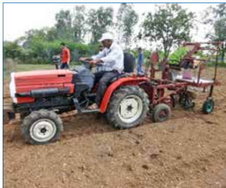
Automatic vegetable transplanters for vegetable seedlings developed at Maharana Pratap University of Agriculture and Technology (MPUAT), Udaipur (left) and Mahatma Phule Krishi Vidyapeeth (MPKV), Rahuri (right)
