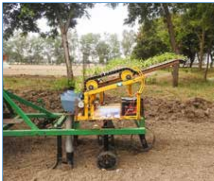
Automatic vegetable transplanters for vegetable seedlings developed at Maharana Pratap University of Agriculture and Technology (MPUAT), Udaipur (left) and Mahatma Phule Krishi Vidyapeeth (MPKV), Rahuri (right)
