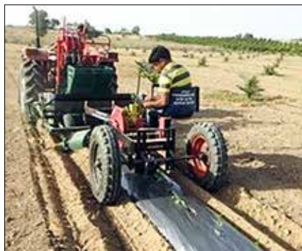
Tractor drawn semi-automatic vegetable transplanter for vegetable seedlings developed at Punjab Agricultural University, Ludhiana (left) and Maharana Pratap University of Agriculture and Technology, Udaipur (right)
