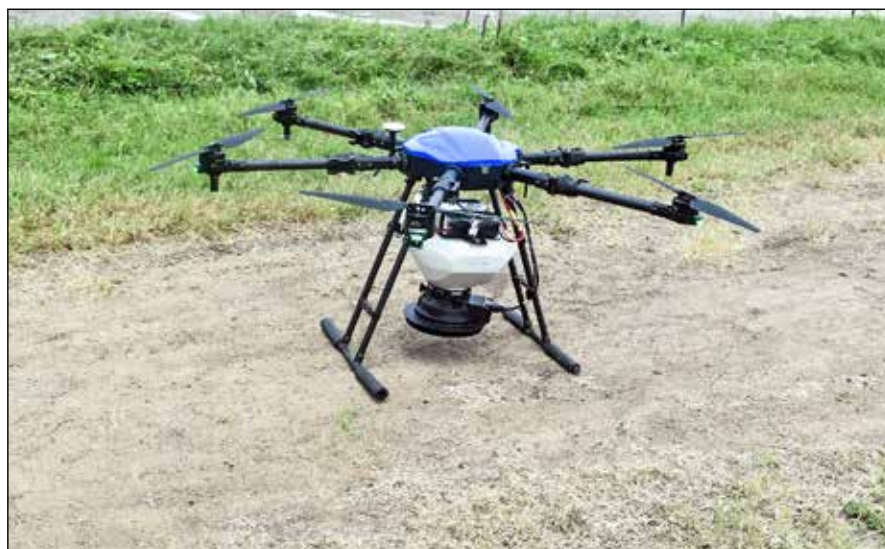
Drone attached with spreader for fertilizer application
