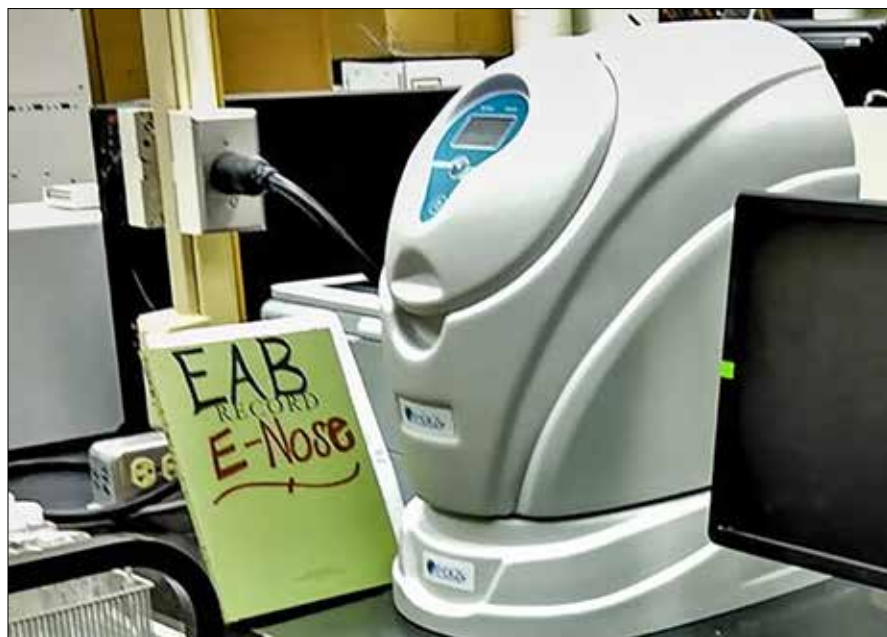
Electronic nose for the detection of Emerald ash borer Source: United States Department of Agriculture
