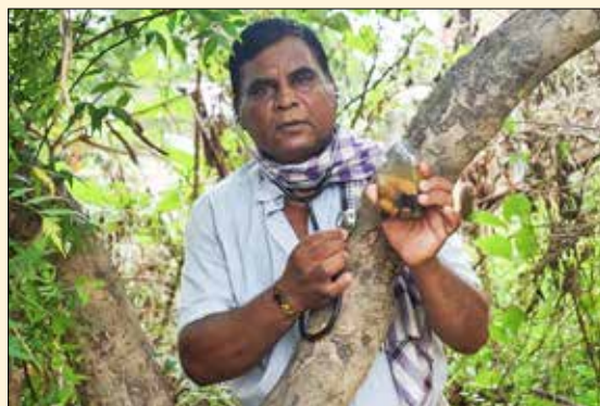
Chakradhar Pradhan, who innovated the early detection of borer pests in trees using a stethoscope
