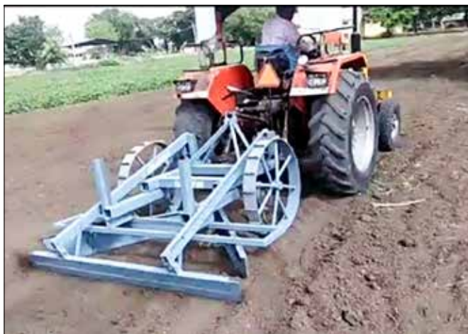
Automatic tractor drawn compartmental bund former
