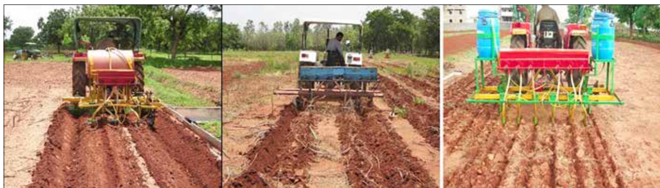
Implements for key to success of Conservation Agriculture practices (a) CRIDA raised bed planter with herbicide applicator; (b) CRIDA zero till planter with ridger; (c) CRIDA precision planter with herbicide applicator
