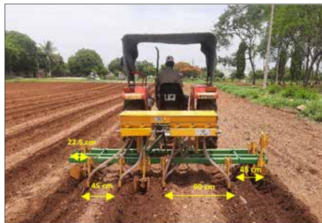
Sowing of pigeonpea + sorghum strip cropping system with 5-row BBF planter
