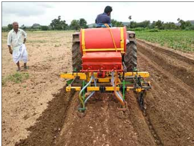
CRIDA variable width raised bed planter cum herbicide applicator
