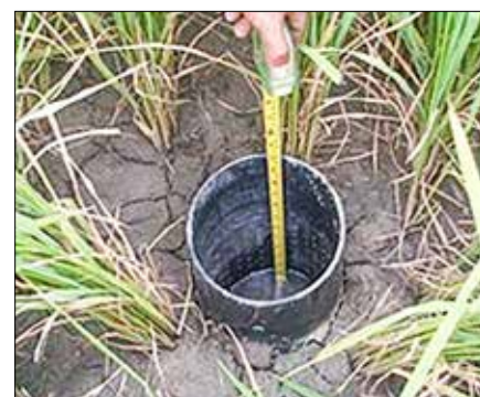
Use of paani-pipe to monitor the water level in rice fields for AWD method of irrigation
