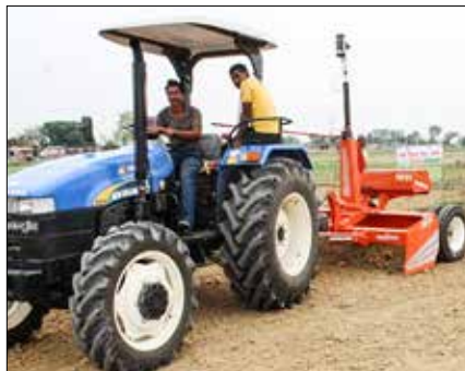
Demonstration of laser land leveling in adopted village Uprama by KVK, Banka, Bihar
