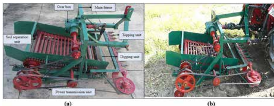
Fig.1. (a) Developed onion harvester with topping unit, (b) working under actual field conditions.
