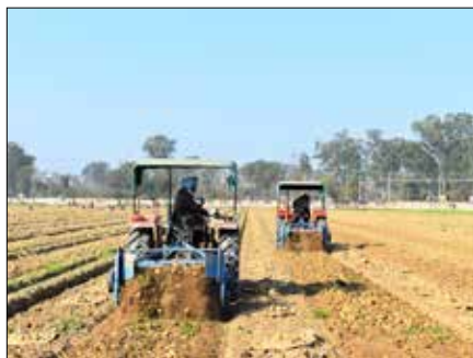
Fig. 5. Potato harvesting with tractor operated digger elevator
