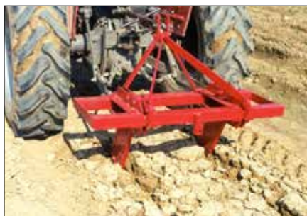
Fig. 1. Deep tillage with subsoiler and rotavator operation for seed bed preparation
