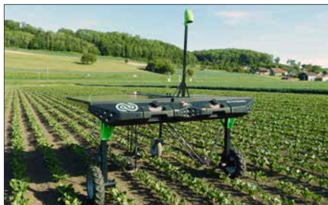
Solar powered weeding robot (Source: Ecorobotix)
