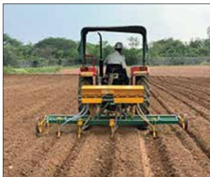
Implement customised for 4:4 sorghum and pigeonpea strip crop sowing
