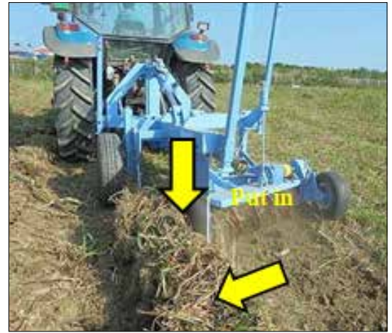
Mechanism of cut-soiler operation for preferential shallow sub-surface drainage construction
