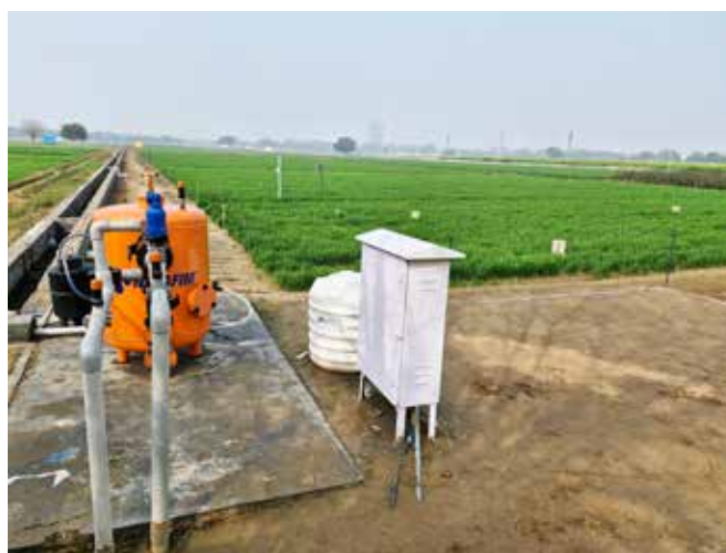
Fertigation through sub-surface drip system (Source: Author's research field)
