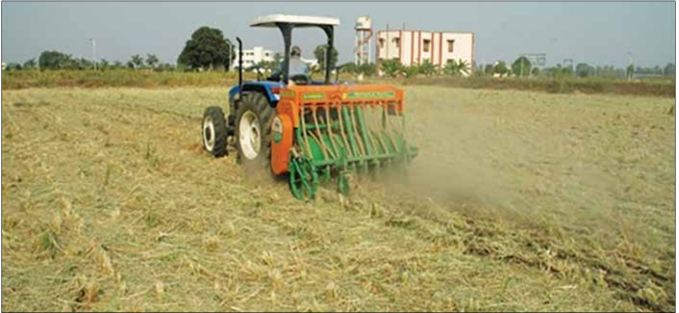
Wheat sowing in rice residues with Happy seeder
