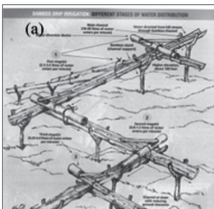
Bamboo irrigation system (a) and Zabo (b) system of water management in northeast India (Source: Bundela 2007, Singh et al. 2018)
