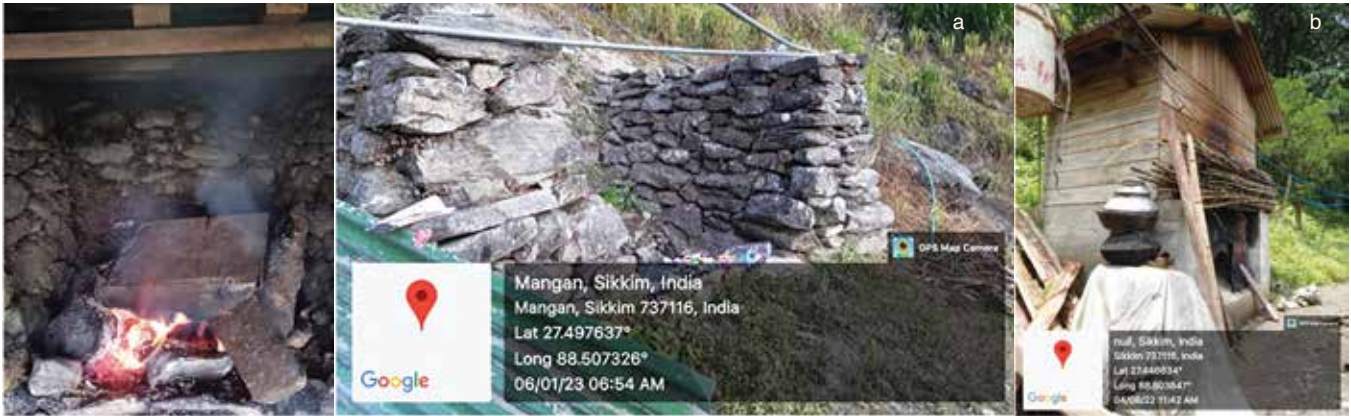
Combustion drying of large cardamom in (a) Traditional and (b) Improved bhattis at Dzongu, north Sikkim
