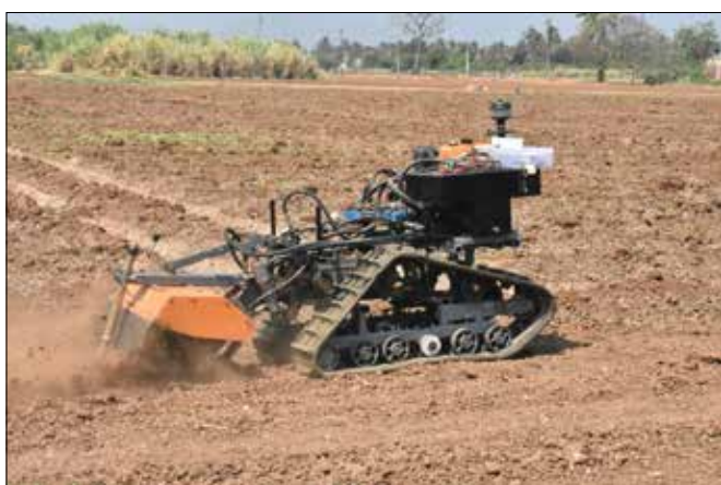
Self-propelled track type vehicle for small farms for tillage
