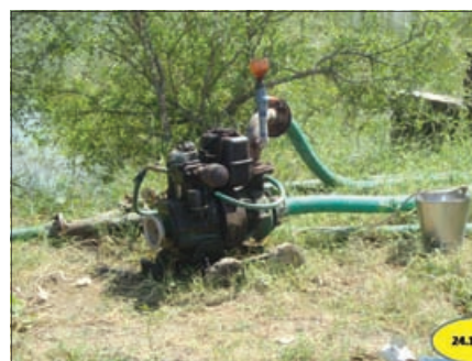
Water is pumped using diesel or electric pump from the water harvesting tank
