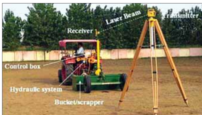
Fig. 2. Part of laser land leveller
