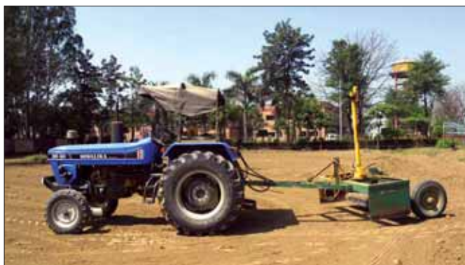
Fig.1. Laser land levelling in the field
