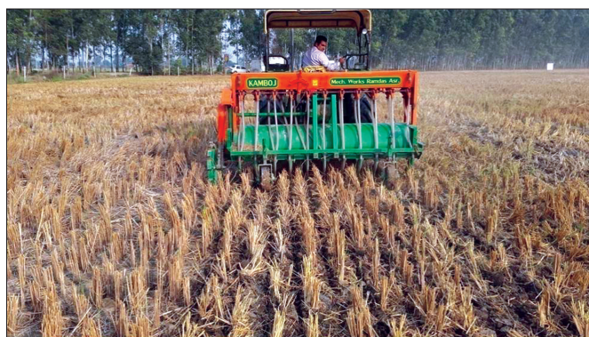
Fig. 2. Turbo Happy Seeder for seeding in to loose crop residue
