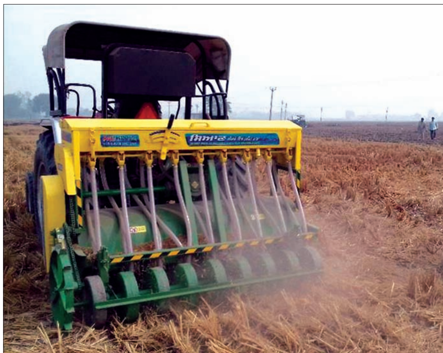
Fig. 1. Happy seeder machine directly sowing wheat into heavy paddy
