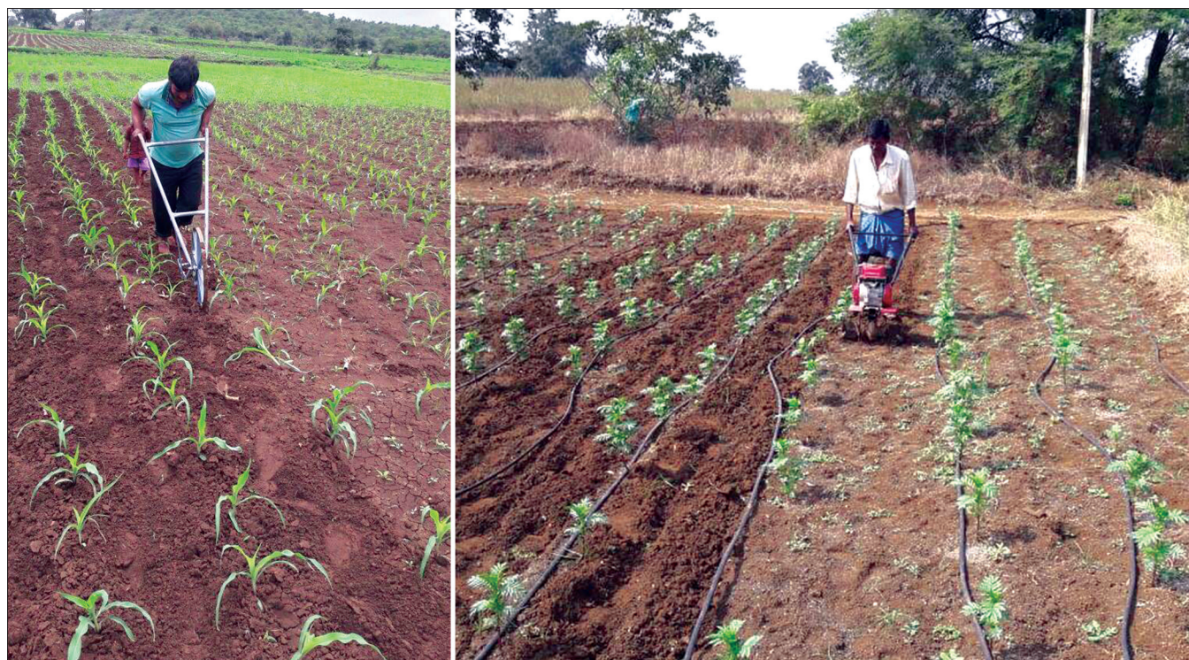
Fig. Weeding operation by farmer with wheel hoe and self-propelled weeder
