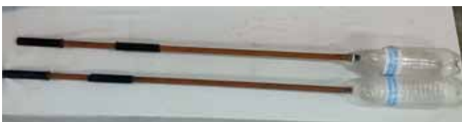
Single use Plastic bottle handmade Fruit plucker/harvester
