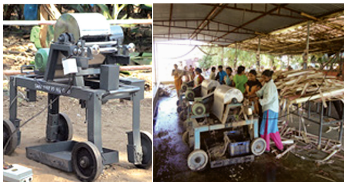
Extraction of fibre from pseudostem
