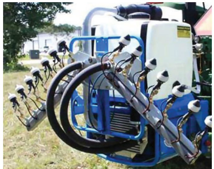
Electrostatic sprayer for orchard (Imported and marketed in India by Eco Agro services)
