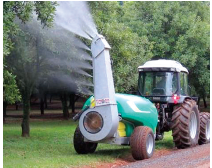
Centrifugal fan sprayer (JS Drive Engineering, Malaysia)
