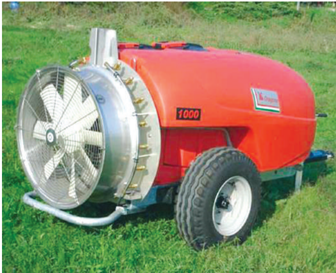
Axial fan air assisted sprayer (Dragone Company, Italy)
