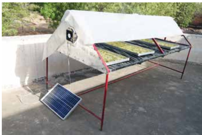
Sangri drying in CIAH solar drying structure
