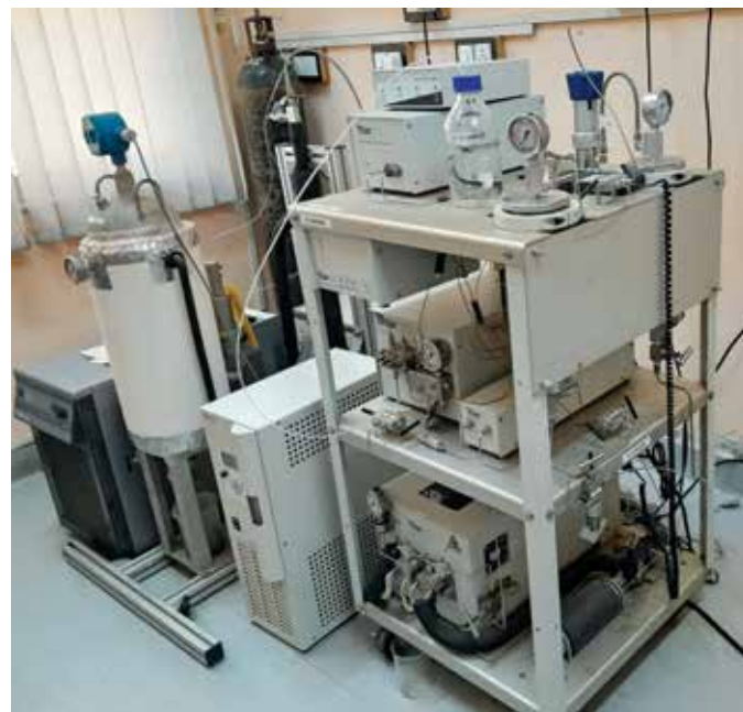
Fig. 3. Super critical extraction facility at ICAR-DMAPR, Anand
