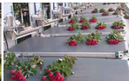
Cleaning, grading, sorting and packing combo machine (Source: http://www.sonerkazaz.com )
