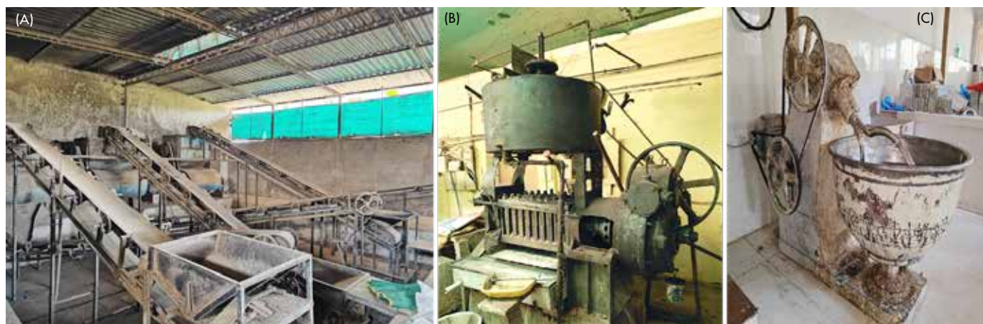
Kokum butter processing traditional equipment for (A) Seed decortication, (B) Oil extraction, and (C) Butter clarification
