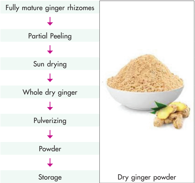
Process flowchart for production of dry ginger powder
