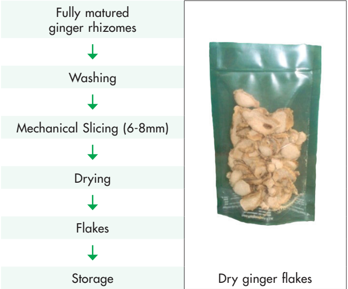
Process flowchart for production of dry ginger flakes
