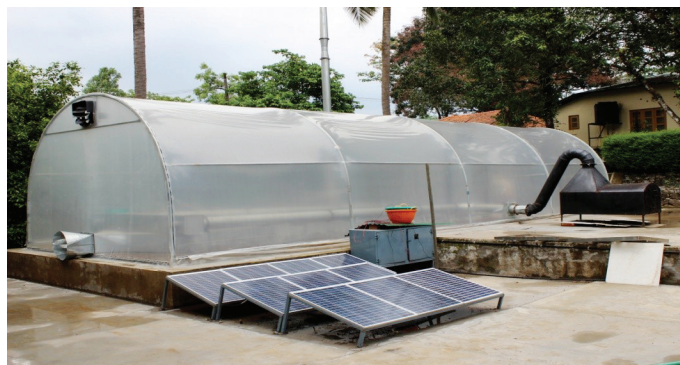
Solar tunnel drier of size 12 × 4 m
