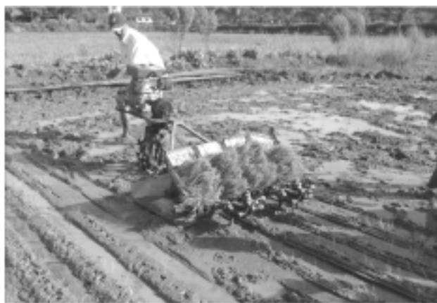
Fig. 3. Four row self propelled transplanter operating in the field
