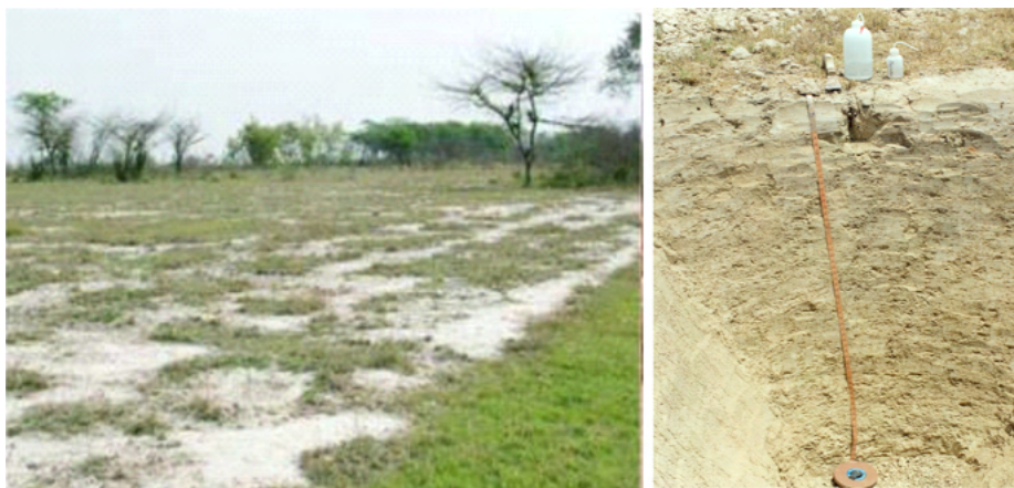
Fig. 3 Typical sodic soil at the Bichian experimental site (left) and soil profile (right) showing kankar -calcic ( \text{CaCO}_3 ) layer
