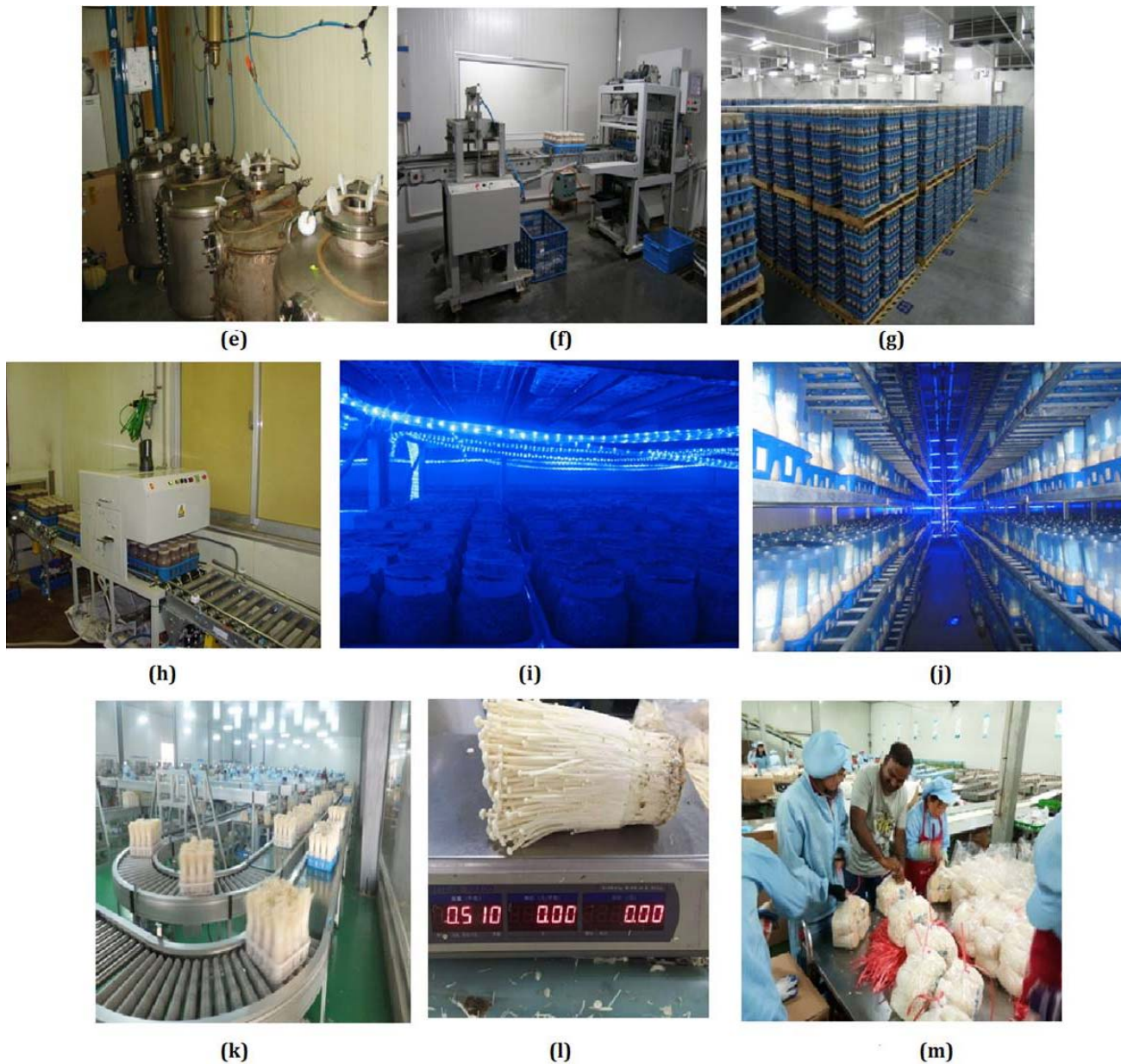
Fig.7. F. velutipes cultivation in an automation mode (a. Substrate filling machine; b. PP bottles with filled substrate; c. Staking of substrate filled PP bottles for sterilization; d. Large scale autoclaves for substrate sterilization; e. Liquid spawn facility; f. Inoculation of substrate with liquid spawn; g. Incubation of spawned substrate; h. Scratching of substrate for fruiting initiation; i. LED lighting with blue lights for uniform fruiting; j. Fruiting initiation under controlled growing conditions; k. Shifting of fruiting trays using conveyer system; l. Harvesting of fruiting bunches with uniform weight and quality; m. Packing of fruiting bunches for sale
