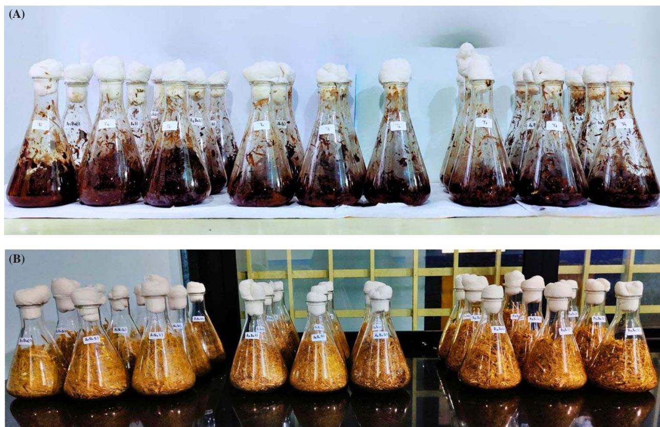
Fig. 1. Efficacy of consortia for degradation of different SMS in flasks. (A) Treatment flasks at day 0. (B) Treatment flasks at day 80
