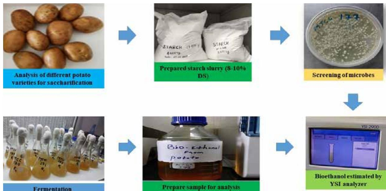
Figure 1. The bioethanol production process from potato
